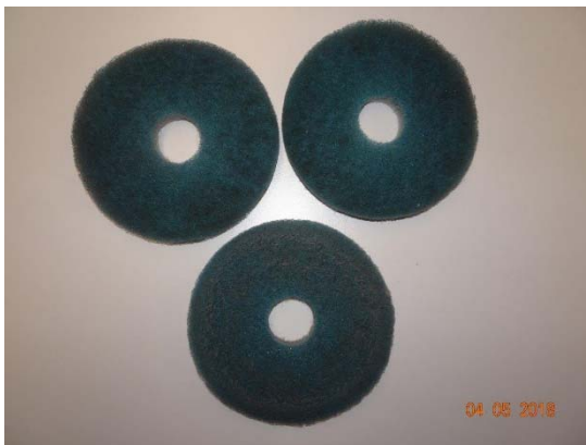
Abbildung 211: WNG ID 920: Zuluftfilter
