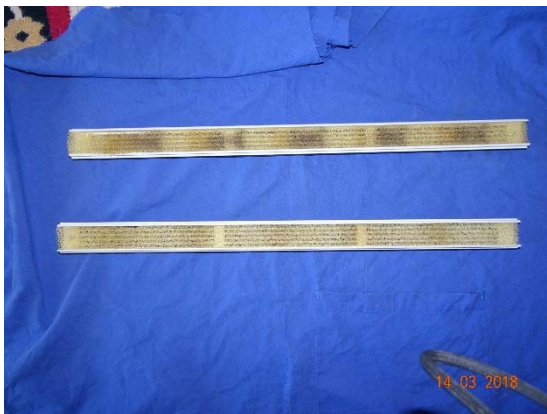
Abbildung 192: WNG ID 820: Zuluftfilter
