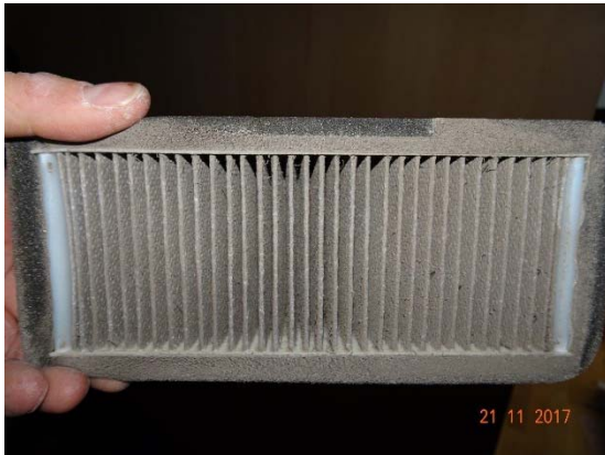
Abbildung 21: WNG ID 110: Zuluftfilter
